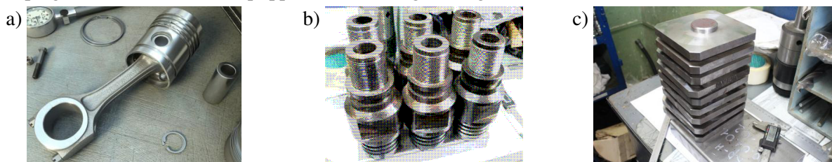
Fig. 1. Controlled spare parts: a – connecting rod and piston group YAMZ-236HM2; b – adapter 122.21.00.00.008-02; c – insert 1222.05.08.00.001
